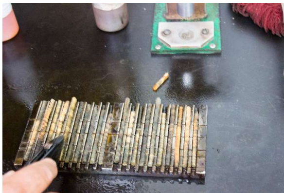
Figure 8: Removing the red parts indicating the heartwood on the core samples
