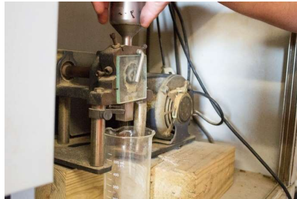
Figure 13: Grinding the core samples for the X-ray measurement
