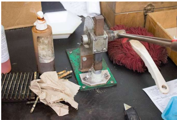
Figure 14: Compressing the ground core samples into the measurement cup for X-ray measurement
