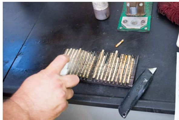
Figure 9: Spraying the indicator for copper on the core samples
