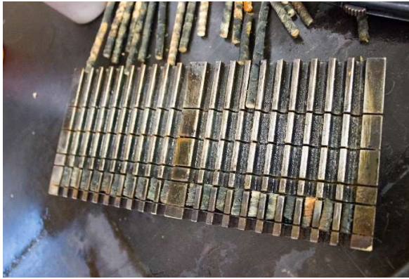
Figure 10: Cutting the samples on a size of 0.6 inches
