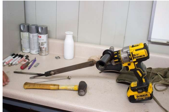
Figure 7: Drill to make core sample borings
