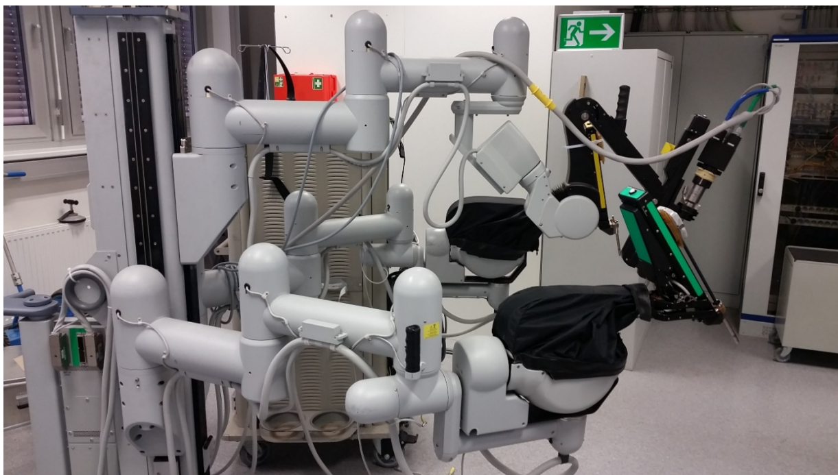
Figure 1. The first-generation da Vinci Surgical System patient-side cart features two robotic arms for manipulating surgical instruments and one robotic arm for controlling an endoscope camera.
