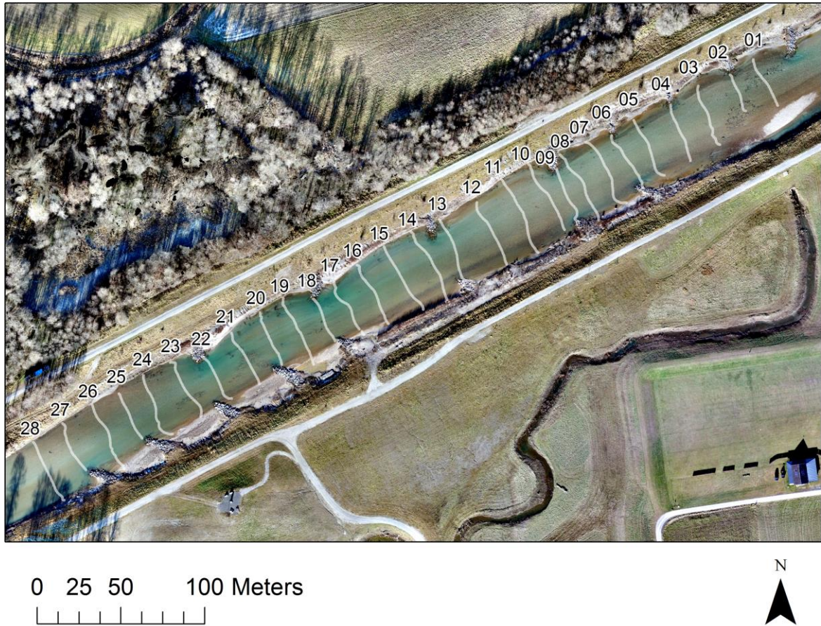
Fig. 28 Location of echo sounding samples acquired at cross sections of the Gail on the 09.12.2015 at approx. 20m intervals.
