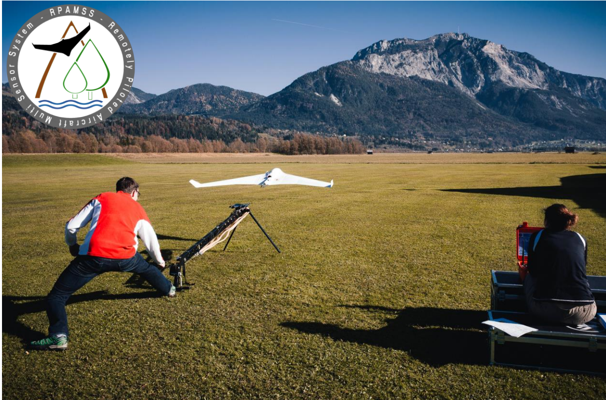
Fig. 1 The C-ASTRAL Bramor UAV taking off at the Feistritz study site. The fixed wing platform is launched by catapult and auto piloted during the entire flight by communication to the ground station, which is visible on the right.
