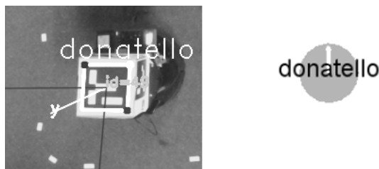
Figure 5.5: The left side shows the image from the top mounted camera and the drawing of the detected marker. The right side shows the visualization of the resulting pose in Rviz.
