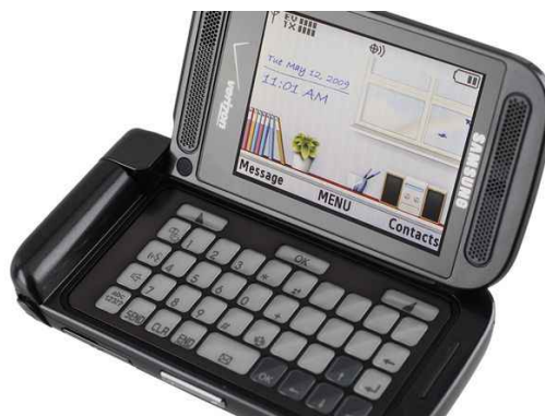
Figure 4.14 Samsung Alias2 SCH-u750 with adaptable e-paper keyboard. (German, 2009)
