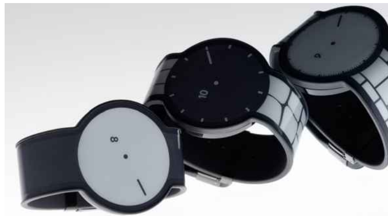
Figure 4.12 Sony FES Watch U with ePaper watch face and wrist band. (Lamkin, 2015)
