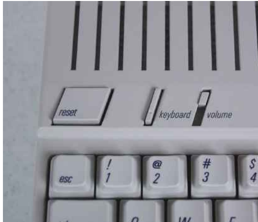
Figure 3.3 Switch on Apple IIC computer keyboard to switch between the QWERTY and an virtual DVORAK layout. (Vectronic's, 2009)
