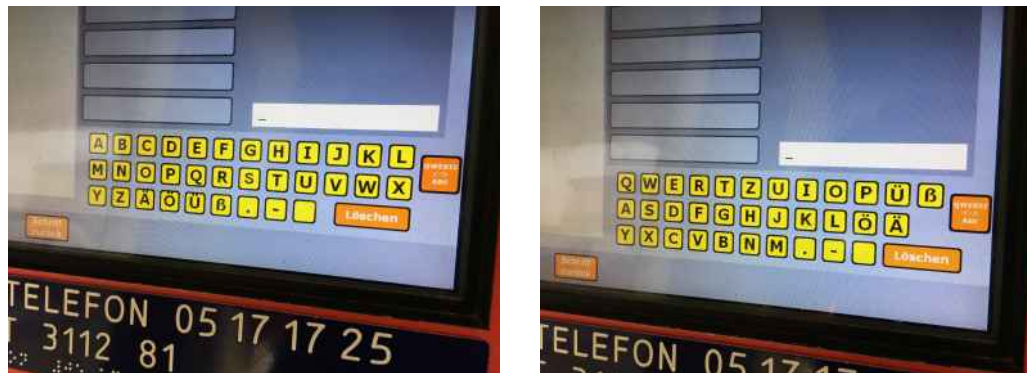
Figure 3.5 Ticket machines off he ÖBB, being able to switch between an alphabetic (left) and the QWERTZ (the German equivalent; right) layout.
