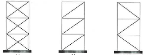
Figure 23 – types of concentric bracing 55
