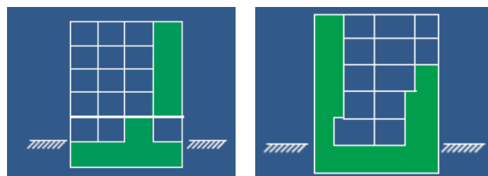
Figure 17 – interrupted load path of lateral-resisting-elements 42
