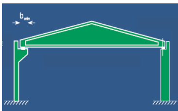
Figure 30 – support connection of prefabricated elements 72
