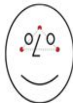
Figure 13b (1b). Shows the placements of three EOG electrodes to record eye movement. The three EOG electrodes will be positioned at the corners of a right-angled triangle; which legs of the triangle from two spatially orthogonal components. The corresponding bipolar EOG components will capture both horizontal and vertical EOG components. The electrodes are positioned close to the eyes to minimize the influence of non-EOG components .
