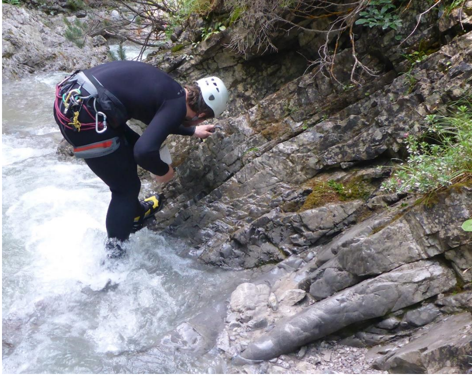
Figure 1: The author measuring the strike and dip of joints formed by bedding in limestone.
