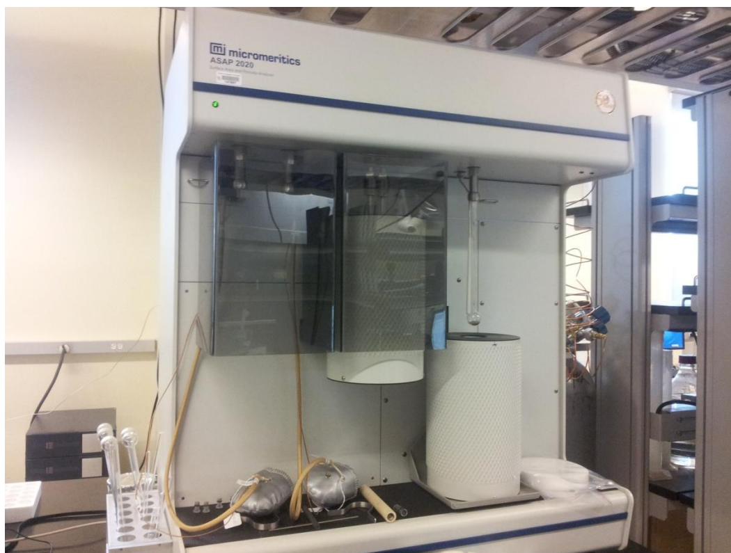
Figure 6: BET instrument Micromeritics ASA 2020 in the UD Material Science Lab
