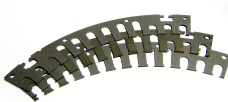
Figure 10: The stators are made out of laser-cut iron sheets
