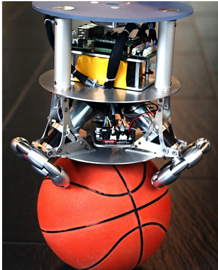
Figure 6: Omniwheels with different radii, as seen on the FHS-ballbot [5]
