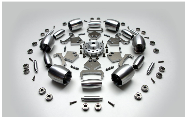
Figure 2: A disassembled omniwheel of the FHS-ballbot. It has 12 separate rollers. Number of parts: 78, [5]
