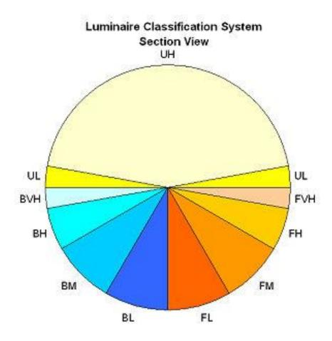
The Luminaire Classification System Section View provided by IES displays the zones referenced in LCS and BUG ratings. These zones are comprised of three main categories; Forward Light (FVH, FH, FM and FL), Backlight (BL, BM, BH and BVH) and Up Light (UL and UH.) The subcategories are used to provide more thorough analysis of light distribution.
