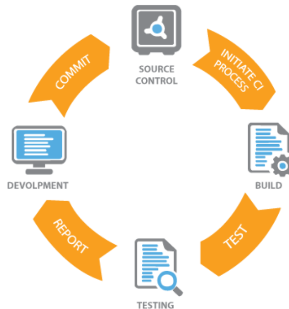
Figure 2.1 - Continuous Integration process (Hirt, 2015)
