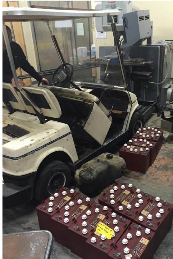
Figure 5.2 The cart with the batteries supplied by NMHG
