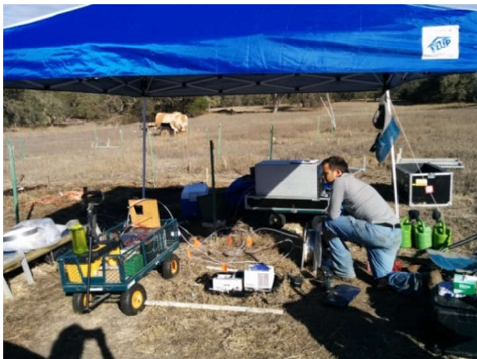
Figure 2: Experimental plot with instrumentation for soil gas flux and nutrient measurement. Left, cart with chemiluminescence NO analyzer and infrared CO 2 analyzer; back, Off-axis ICOS N 2 O laser; right, mobile gas flux chamber being vented in preparation for the next measurement; center, microdialysis set-up with pump and fraction collector and 4 microdialysis probes.
