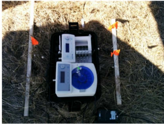
Figure 5: Set-up of the microdialysis system. On top the CMA 400 pump, on the bottom the CMA 470 refrigerated fraction collector. Orange flags mark positions of the membranes.
