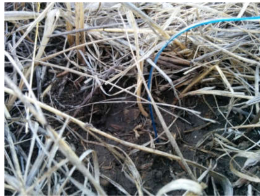
Figure 6: Microdialysis membrane inserted into the soil and connected to an inflow tube (blue, contains MilliQ water) and an outflow tube (white, contains dialysate with soil nutrients).
