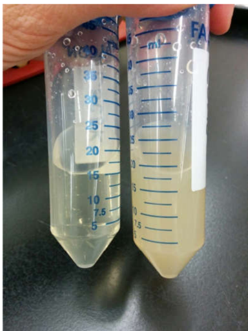
Figure 7: Water extracts before (right) and after (left) filtration with 0.45 celluloseacetate filters. The cloudy brownish color originates from the high clay content of the soil.
