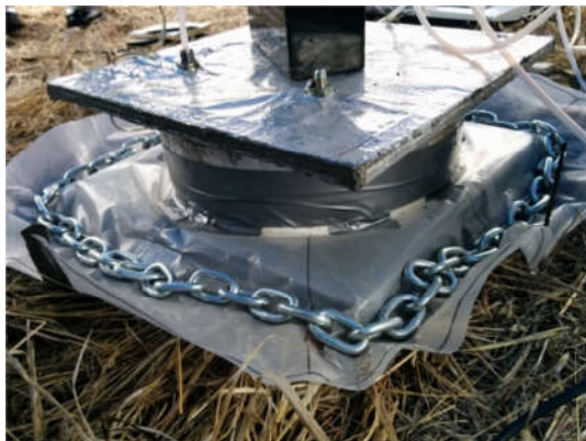
Figure 3: Mobile flux chamber for trace gas measurement. The plastic 'skirt' is weighed down with a heavy chain to prevent lateral in-blow of wind.
