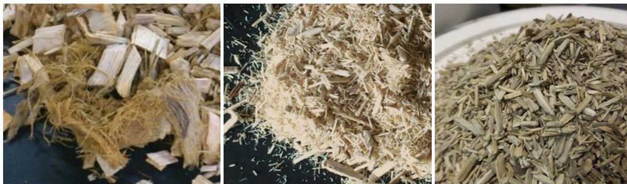
Figure 5. Coarse eucalyptus chips with impurities (left), milled material after hammer mill (middle) and screened feedstock (right).
