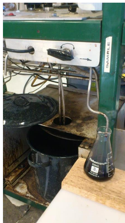
Figure 9. Reactor main outlet with pot and bypass for sample taking.
