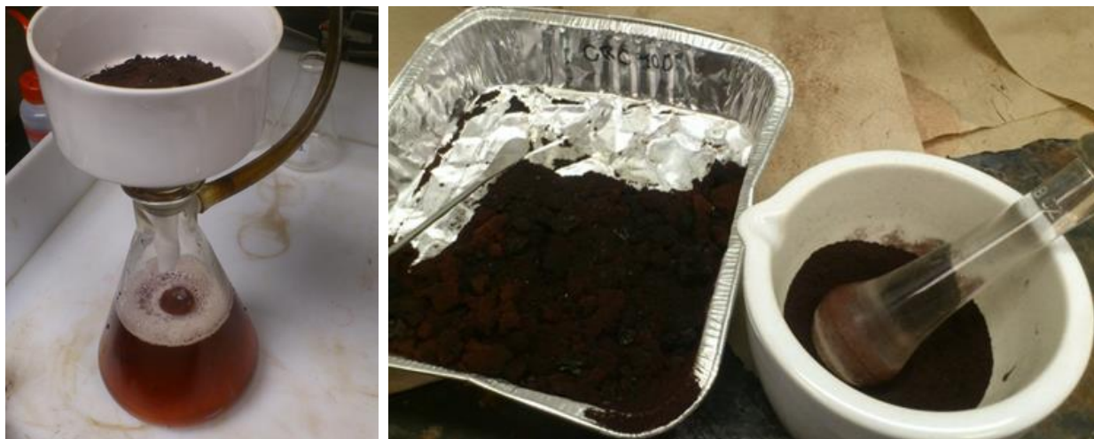
Figure 10. Buchner filtration of the lignin (left) and dry lignin powder (right).
