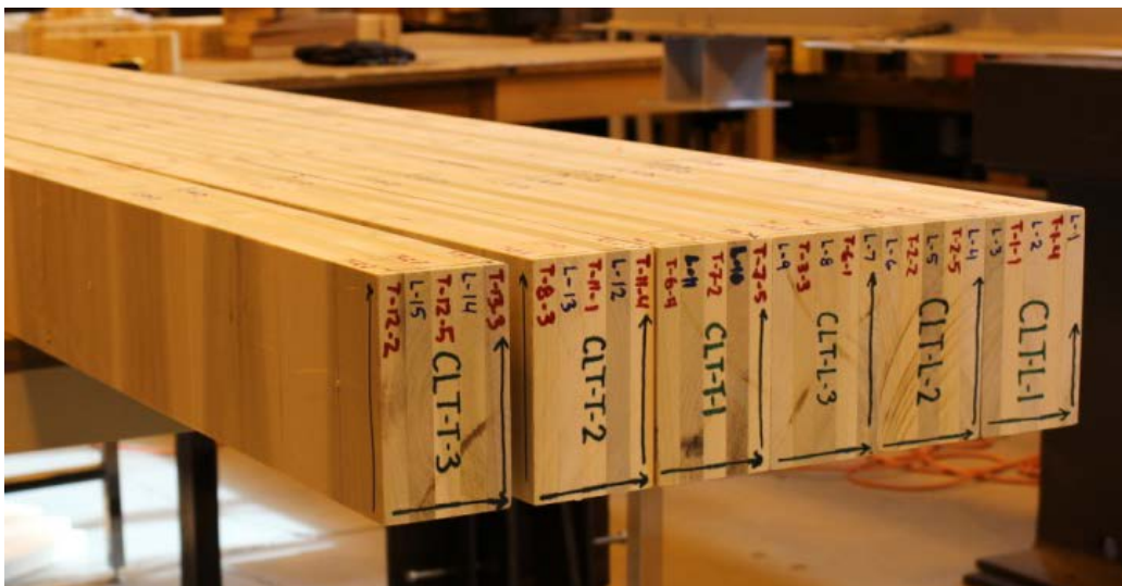
Figure 73: 5-layer CLT from yellow poplar feedstock at Virginia Tech (Beagley et al., 2014).
