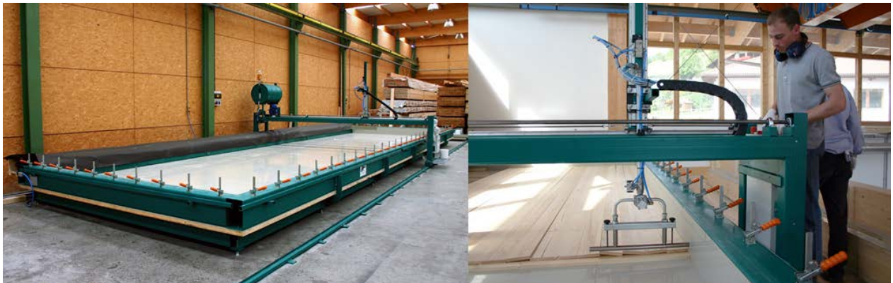
Figure 29: Vacuum press with adhesive application devise (left) adhesive applicator (right). Courtesy of Woodtec Fankhauser
