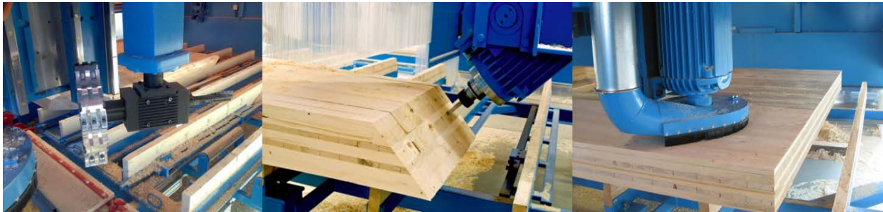
Figure 34: Tools of multiple processing center (B). Courtesy of Hans Hundegger AG
