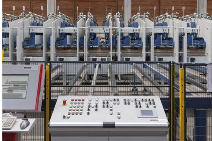
Figure 27 Hydraulic CLT press. Courtesy of MINDA
