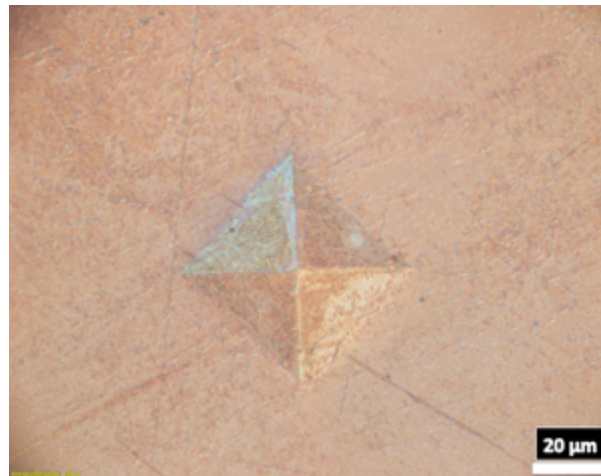
Fig. 4.2: Vickers indent on sx Cu, tested with HV 0.1
