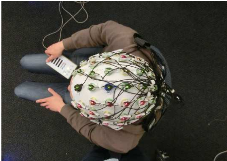
Figure 10: EEG-cap on a subject's head (LED's on each electrode show it's impedance)
