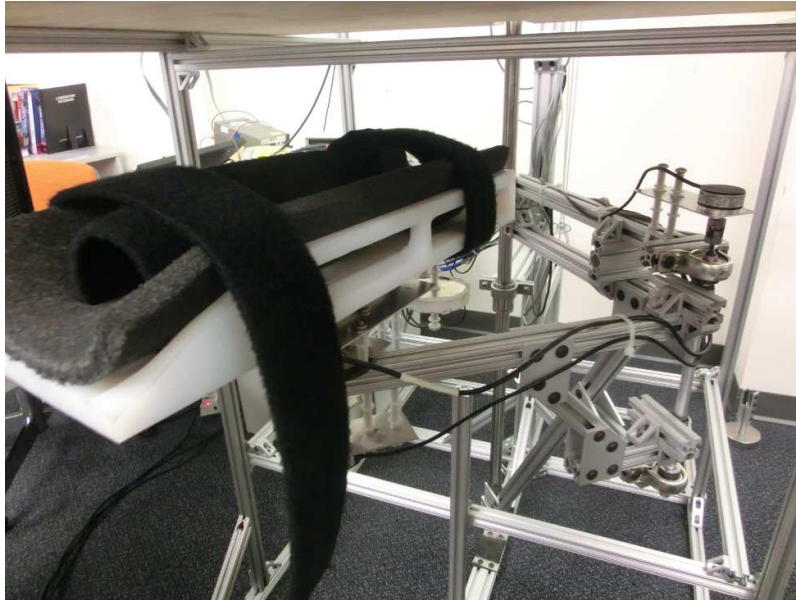
Figure 12: Arm robot system with horizontal screen ( projector is mounted on the ceiling over the system)
