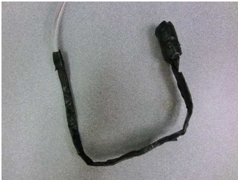
Figure 15: Tendon vibrator after insulation
