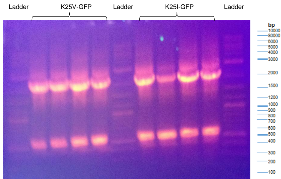
Fig. 8: Picture of a 0.8%-agarose gel with 1% ethidium bromide under UV-light. The samples K25V and K25I showed the expected band at 2000bp and a band at 500bp, which is dispensable.
