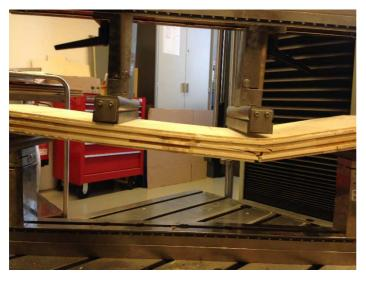
From all this testing we were able to determine that the difference between boards using MUF and UF glue wasn't as important as we originally thought it to be. It was determined that the empty spaces between the pieces of wood (shown in the first picture) was important to the overall strength of the board. Denser boards with less air space performed better than lighter boards with more space. This conclusion makes sense due to having a greater volume of wood and glue bonding available.
