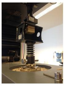
The strength of the actual lightweight boards was done using a three point bending test machine. The test shows if the glue fails before the actual board or vice versa. Below shows the board failing on the right side during the three point bending test. The type of breaking shows that the board failed before the glue bonds.
