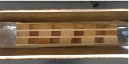
A crucial part of this research was using different types of glue to test the strength of the glue bonds as well. MUF (melamine-urea-formaldehyde) contains lower amounts of environmental toxins than the UF (urea- formaldehyde) glue that was also used. The MUF is desired for use in these panels because it aids in the reduction of formaldehyde emissions.
