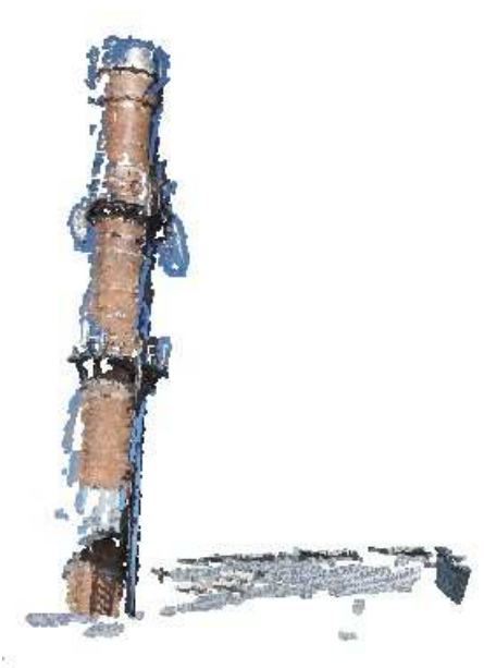
Figure 18: 3D Reconstruction of Chimney from Visual-SFM
