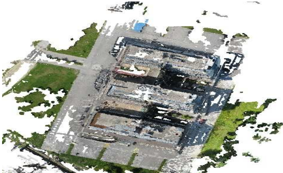
Figure 16: 3D Reconstruction of Intel Mobile Communications Building from Visual-SFM
