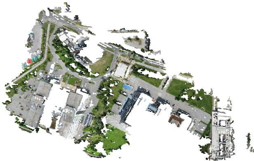
Figure 14: 3D Reconstruction of CUAS Campus, Villach, Austria from Visual-SFM
