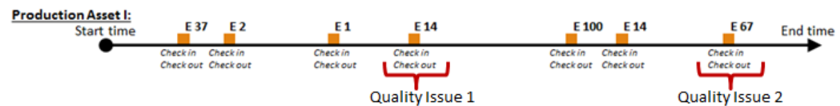
(d) Third Approach - A production asset with two quality issues and how the sub-sequences are defined.
