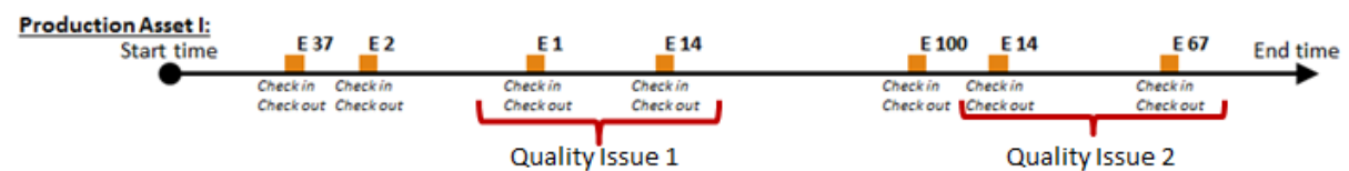
(c) Second Approach - A production asset with two quality issues and how the sub-sequences are defined.
