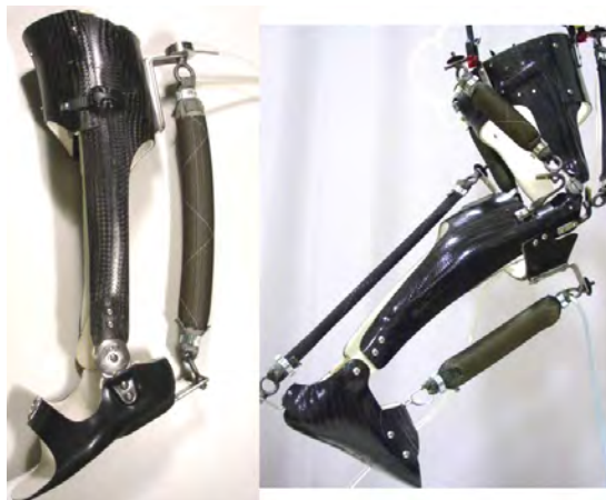
Figure 2.6: Artificial Air Muscle Powered AFO developed at the University of Michigan [Sawicki et al., 2005]
