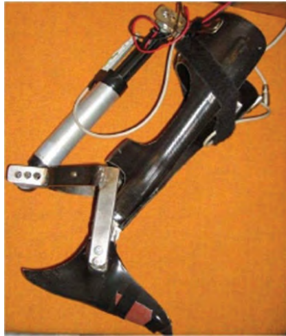
Figure 2.5: MR Fluid Damper Orthosis developed by the University of Halmstad.[Svensson and Holmberg, 2008]
