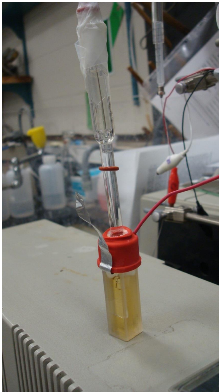
Figure 13 Spectroelectrochemical cell: 1 cm quartz cuvette, ITO working electrode, Pt counter electrode and Ag/ AgCl reference electrode in a reference electrode retainer
