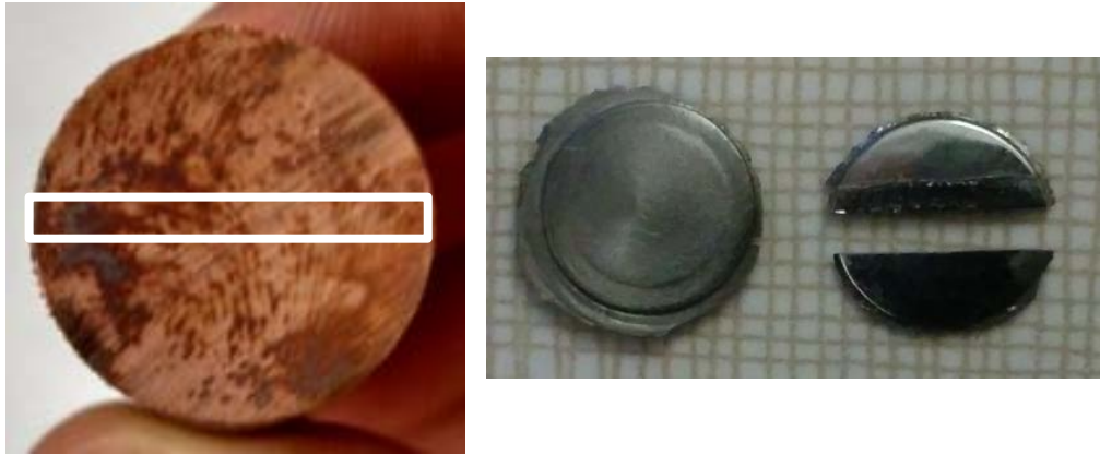
Figure 3.2.1a Illustrations of the ECAP Cu slice and highlighted area from which the bar was cut, left, and HPT PM 2000 disk and where the bar was cut from the center, right.
