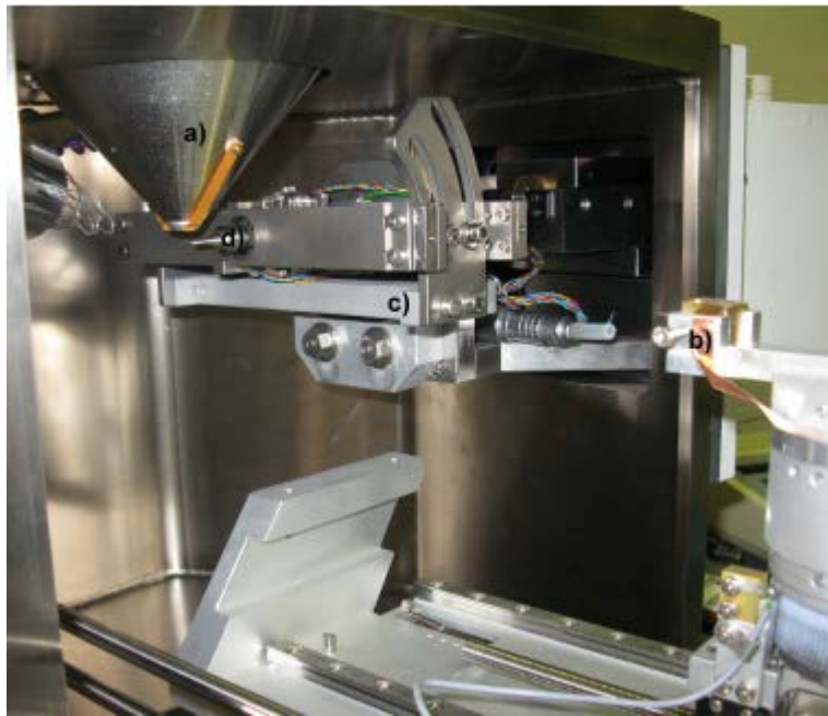
Figure 3.2.4a The ASMEC UNAT SEM II mounted on the chamber wall of the Zeiss Stereoscan SEM 440. (a) is the SEM electron gun, (b) is the xyz moveable SEM sample stage, (c) is the moveable indenter plate of the ASMEC UNAT SEM II, and (d) is indenter head tip
