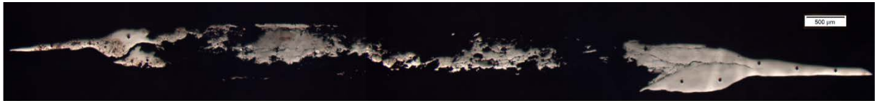
Figure 4.1.2c Optical micrograph of 75-25 Cu-Nb composition ball milled for 40 hours that underwent 5 HPT revolutions. Again the center appears very brittle and a significant amount of material has flaked away.
