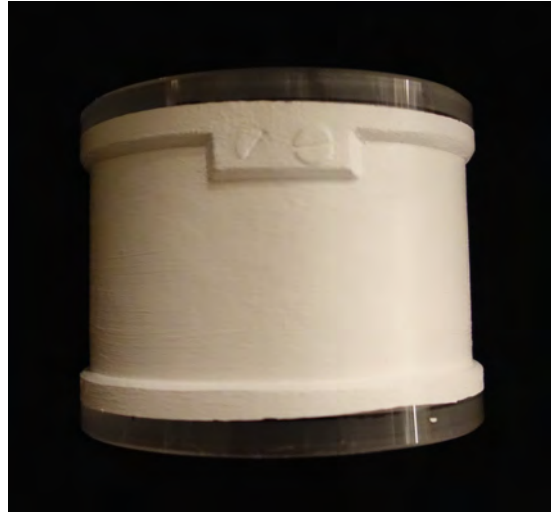
Figure 28: Cell painted with TiO paint
