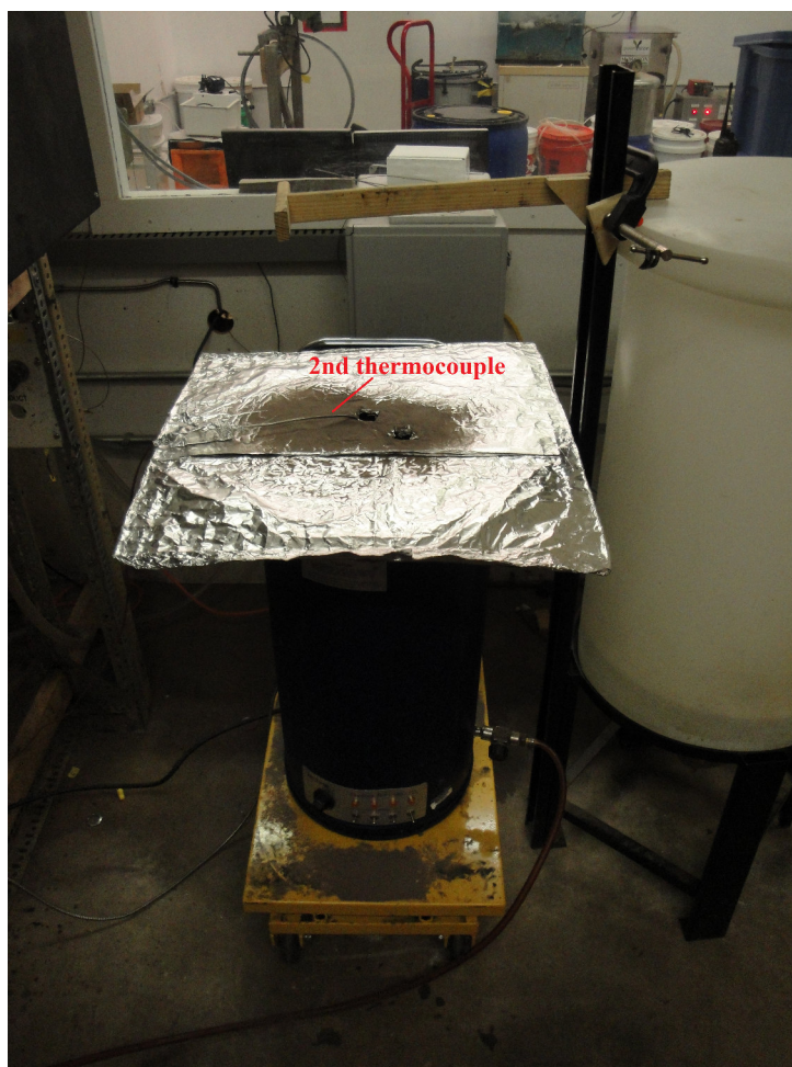
Figure 2.2: Fluidized sand bath.
