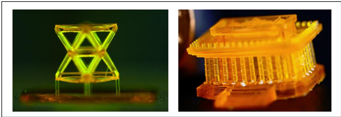
Figure 16: Left: octet-truss unit cell | Right: micro building [mit]
