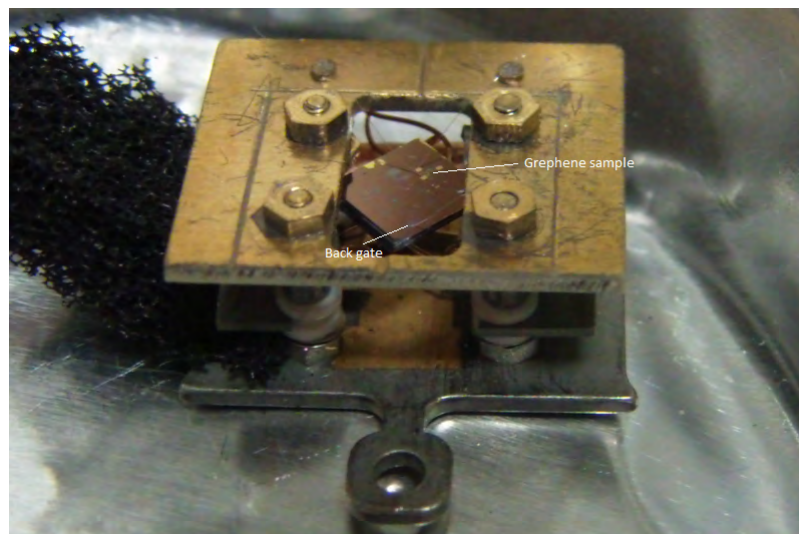
FIGURE 2.8: Sample plate; gold wires were wire bounded to sample plate electrodes; in order to have the back gate, the SiO_2 was scratched for wire bounding
