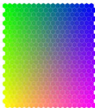
Figure 34: Coloring of SOM neurons based on their topological order in the grid (Vesanto 1999).
