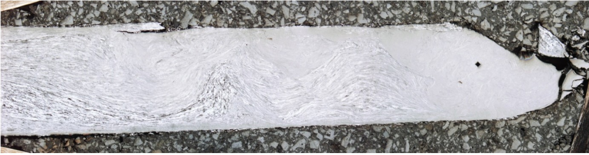
Fig. 4.10: Profile of the heat treated sample #2 ht, showing half of the HPT sample.
