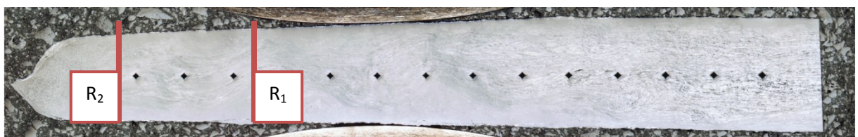
Fig. 4.16: Area for further SEM investigations on the heat treated sample #3 ht.
