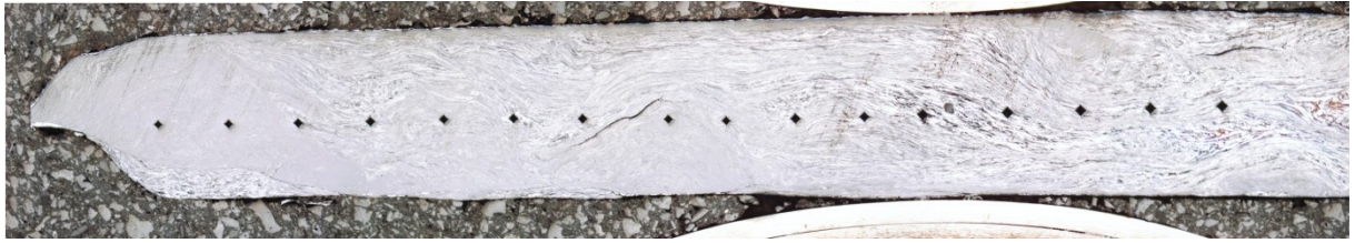
Fig. 4.8: Profile of sample #2, showing half of the HPT sample with microhardness indents.
