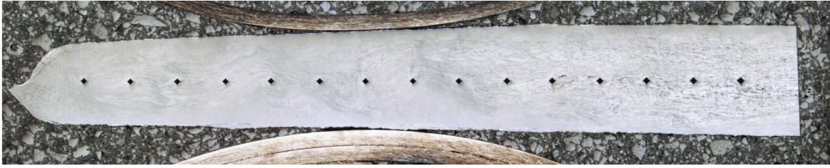
Fig. 4.14: Profile of heat treated sample #3 ht, showing half of the HPT sample with microhardness indents.
