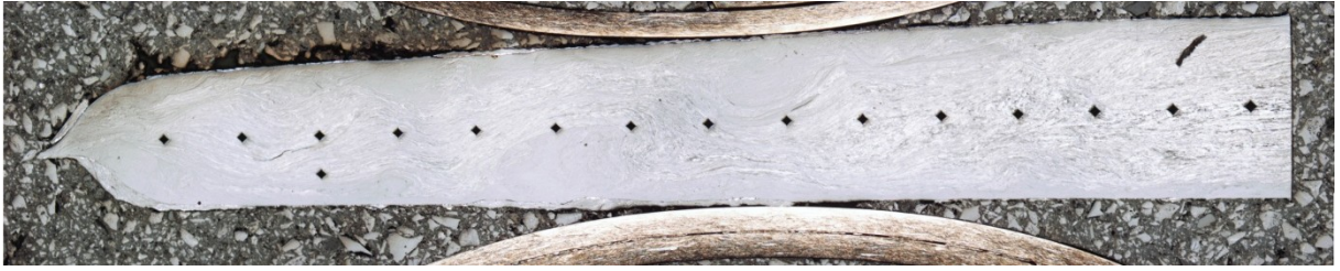
Fig. 4.12: Profile of sample #2, showing half of the HPT sample with microhardness indents.
