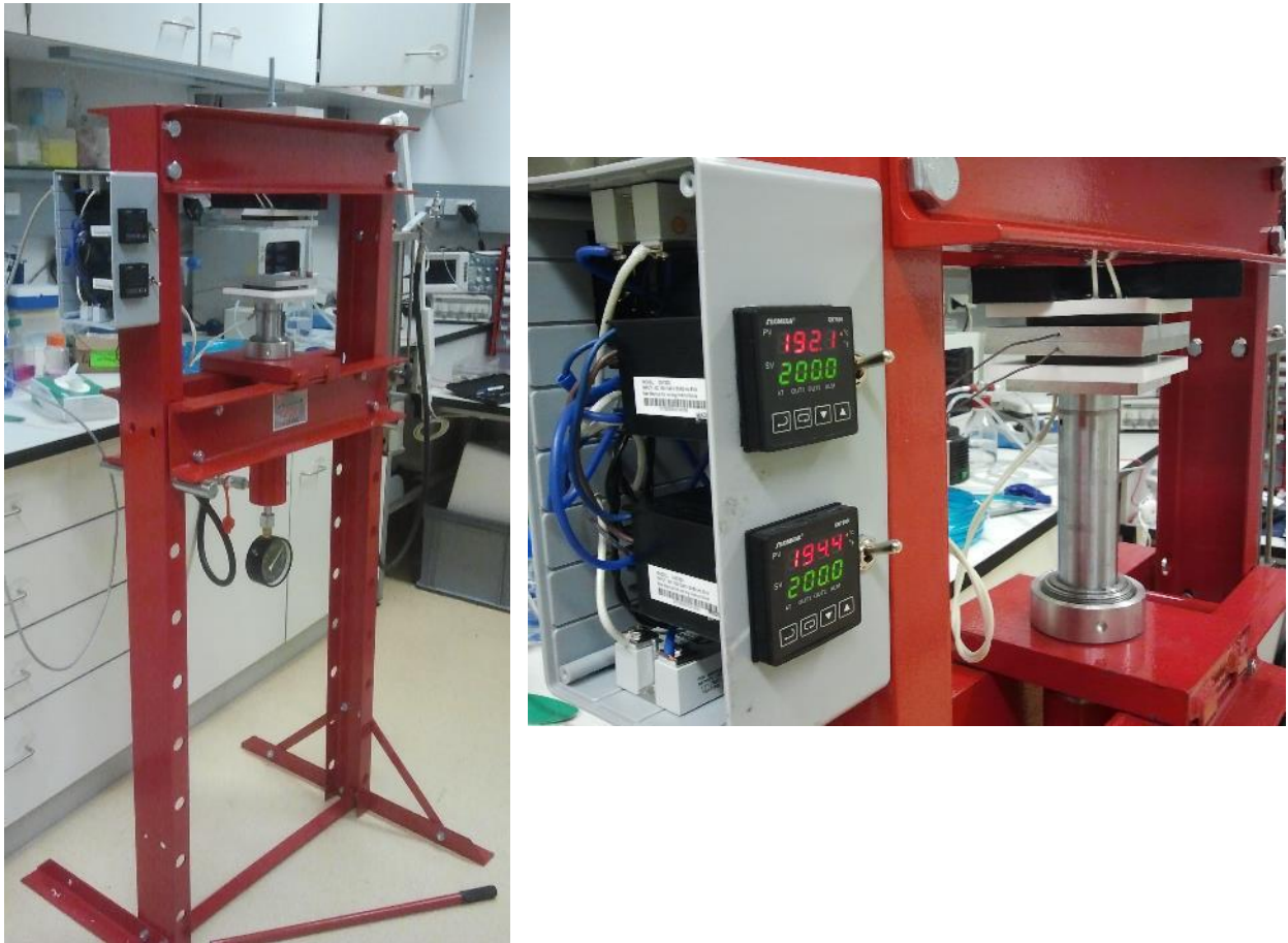
Figure 10. Hot embosser built for the Ertl Lab, shown after assembly (left) and closeup view of the temperature controller and heated platens (right). The frame consists of a 20 ton hydraulic press with heated platens. Temperature is regulated by two independent heaters and temperature controllers (gray box attached to press).
