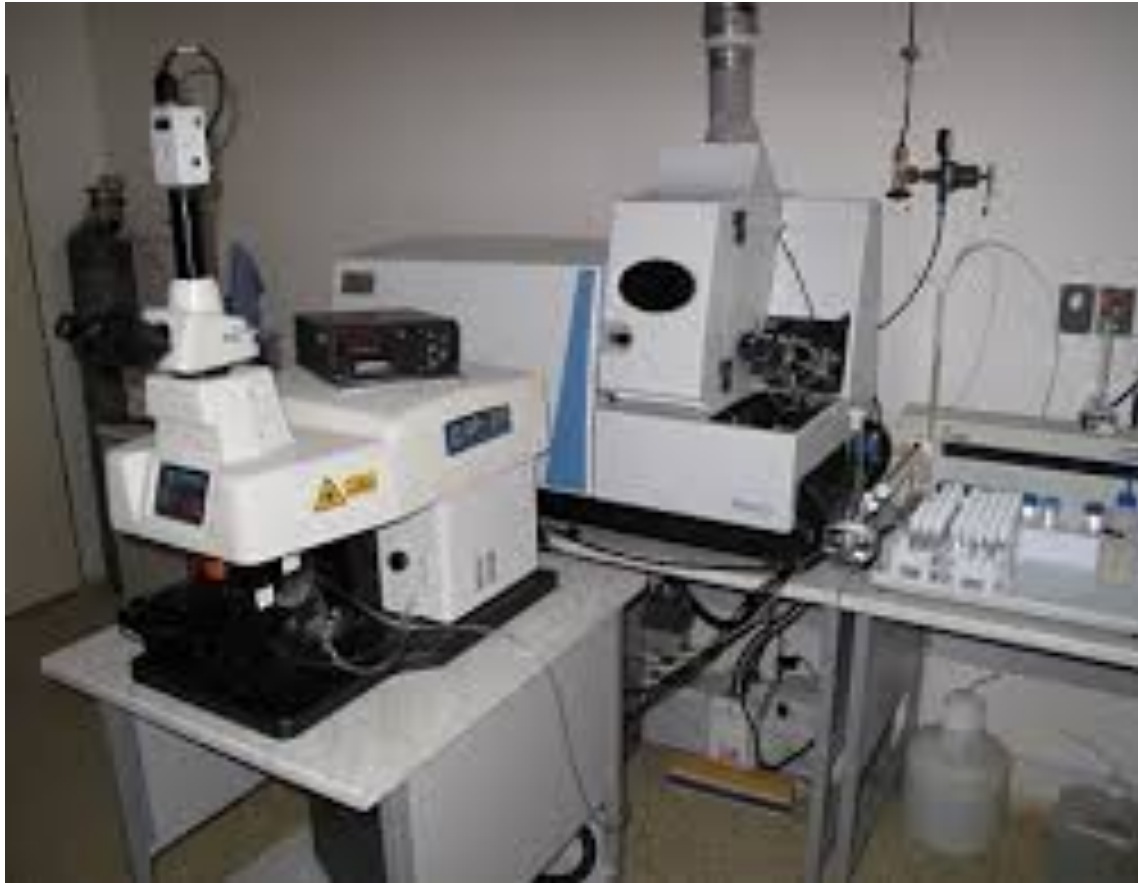
Figure 10: The LA-ICP-MS instrument used in UMass Boston laboratory.
