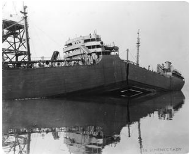
Figure 4: Liberty Ship which cracked in half as a result of a Ductile-to-Brittle Transition
