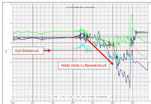
Figure 13 (b) face support pressure drop during stoppage
