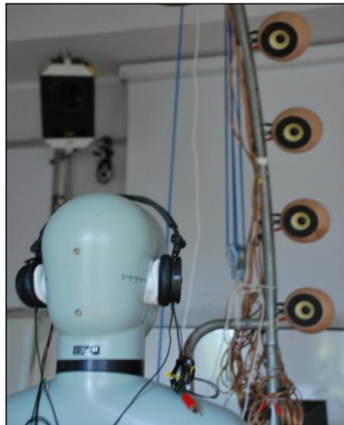
Figure 3.8: Setup to measure the open loop transfer functions for 8 angles of elevation and 12 angles of azimuth.
