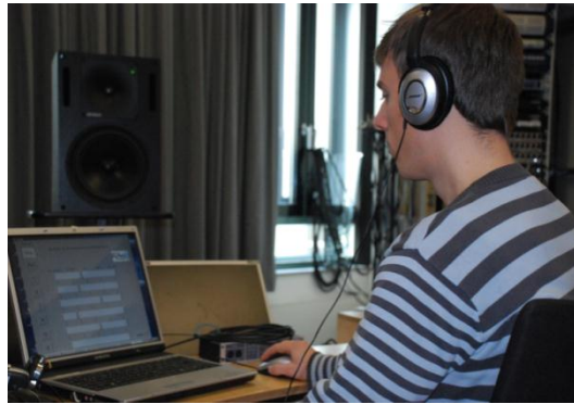
Figure 2.5: Listening test, part II. A test person judges an ANC headphone. The headphones are put onto the test person's head by a tutor, such that the test person cannot recognize the brand of the headphone.
