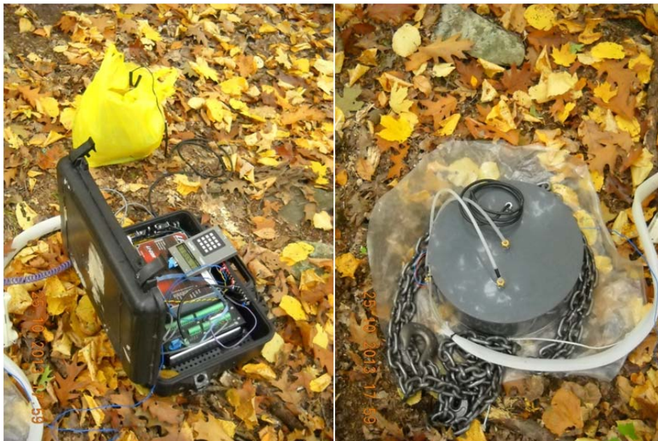
Picture 2: LiCor 6400 portable photosynthesis system (a) adapted with a soil respiration chamber (b) used for respiration measurements in October 2013 at the research site in Black Rock Forest.
