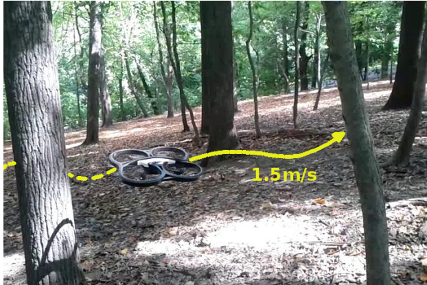
Figure 1: We present a novel method for high-speed, autonomous MAV flight through dense forest areas. The system is based on purely visual input and imitates human reactive control.
