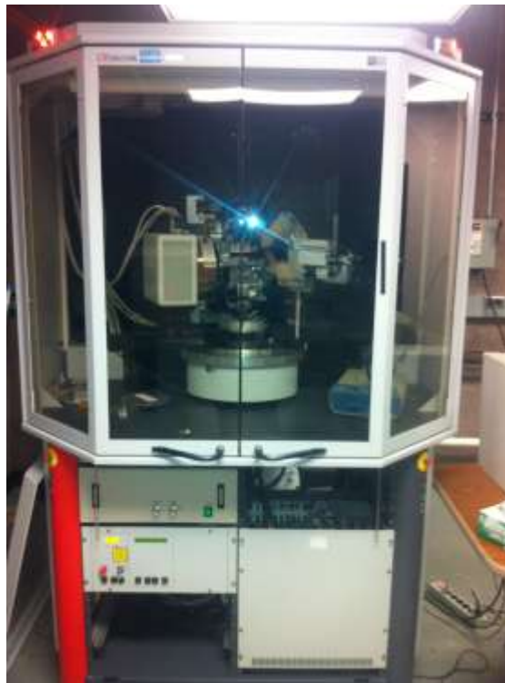
Fig. 3.15 WAXD Bruker AXS D8 Discover (Bruker AXS Inc., Madison, WI, USA)
