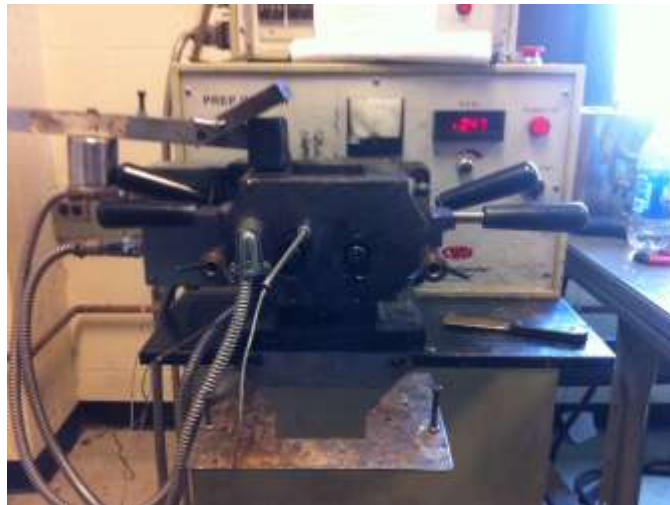
Fig. 3.4 Laboratory kneader Brabender Plasticorder Type PL2000
