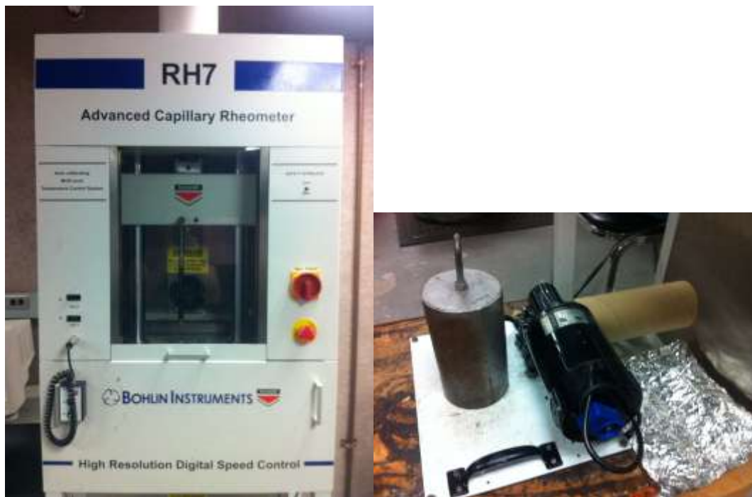
Fig. 3.8 Capillary rheometer (left), home-made take up device with bobbin (right)
