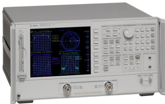
Figure 3.2: 2-port vector network analyzer (VNA) Agilent 8753ES available at the National High Magnetic Field Laboratory (NHMFL) [30]
