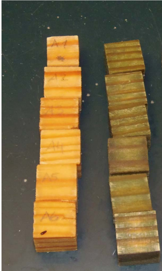
Figure 4: Samples after treatment with borate (left row) and water-borne copper naphthenate (right row)
