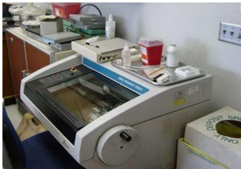
Fig.17 A cryostat can help to overcome conventional obstacles of disinfection since the cold disinfection facilitates complete non-toxic disinfection of the entire cryo-chamber
