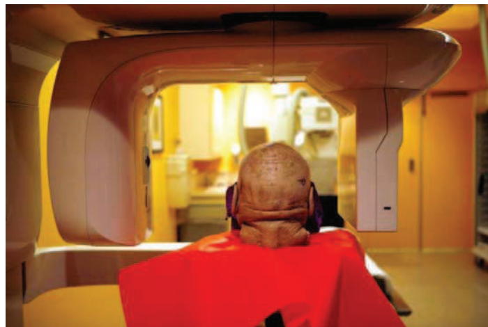
Figure 11 Dental Cone Beam CT Unit with a Flat Panel Detector on the right and the x-ray source on the left. Johns Hopkins Outpatient Radiology Center.
