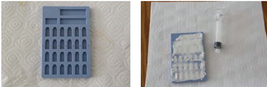
Figure 26 Preparation of bone cement phantoms. A: Silicone mold with surgical absorbable suture. B: Mold filled with bone cement.
