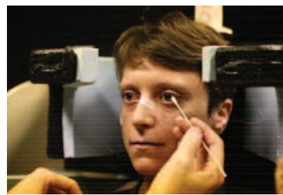
Figure 7 Dual scleral search coil experiment. Left picture: inserting the coil. Right picture: wires coming out of the eyes and adjustment of the coils.
