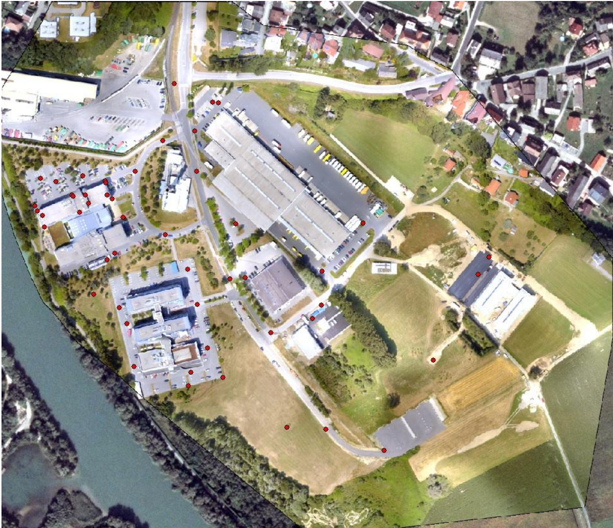
Figure 4 - Bloodhound Orthomosaic over LiDAR Orthomosaic with GPS point (red) reference data
