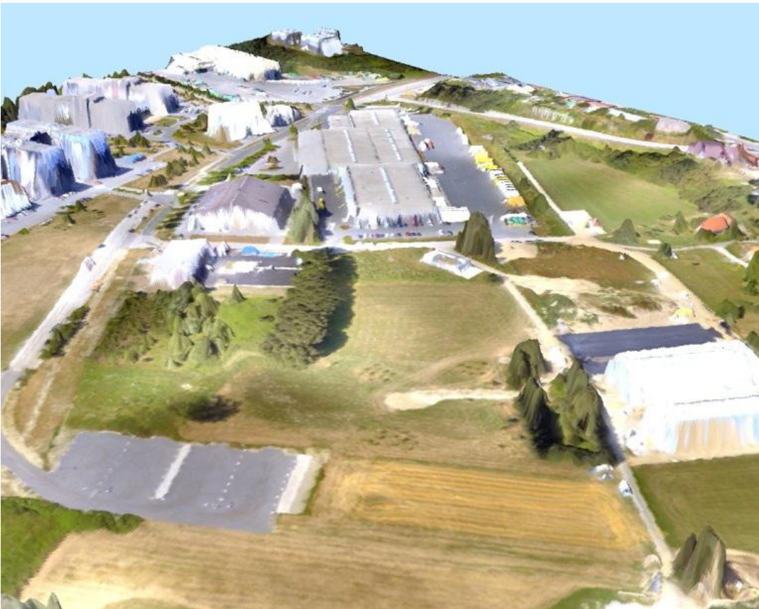
Figure 10 – Bloodhound Orthomosaic rendered in 3D using Bloodhound DSM elevations
