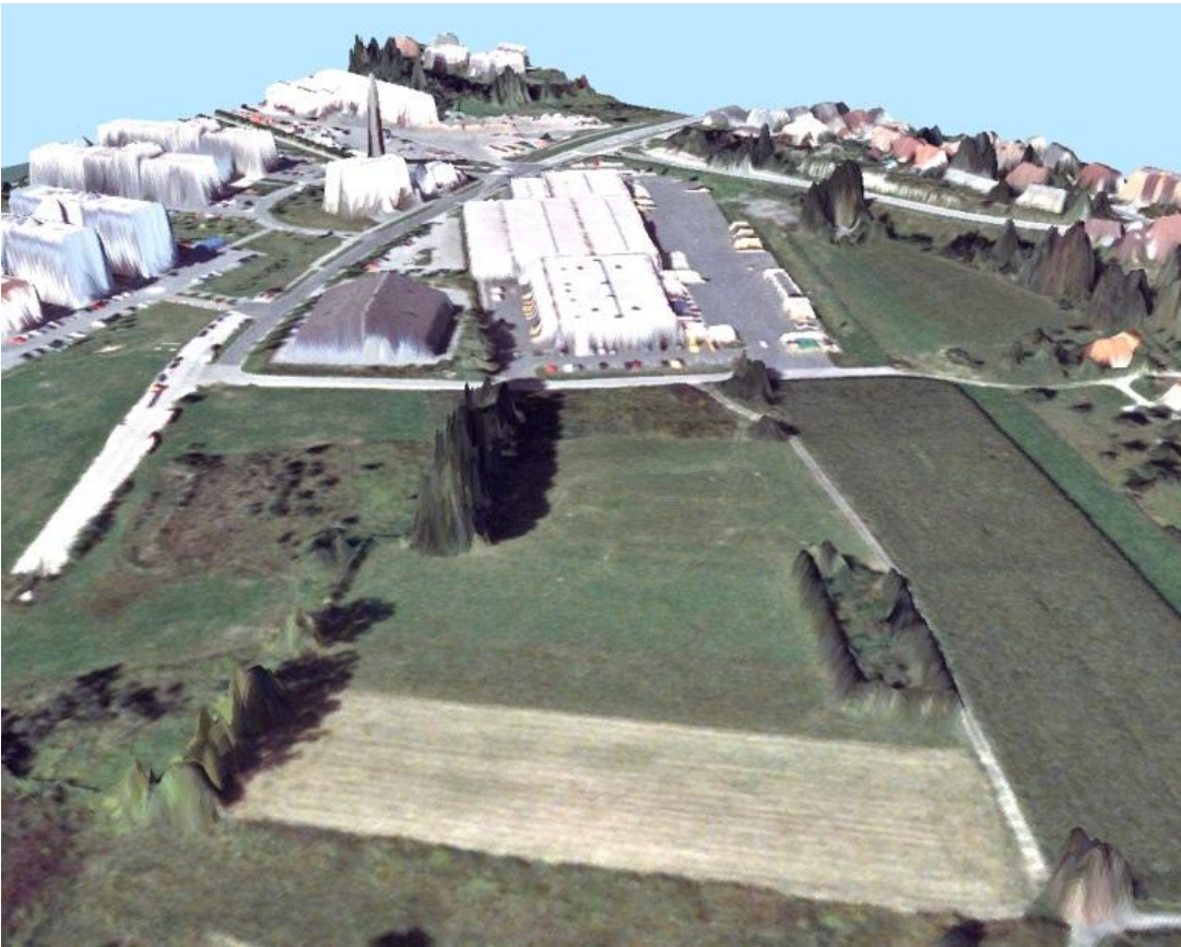
Figure 9 – LiDAR Orthomosaic rendered in 3D using LiDAR DSM elevations
