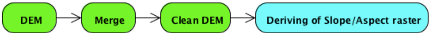
Figure 10 - Schematic representation of the workflow for the DEM processing and the creation of the slope and aspect raster.
