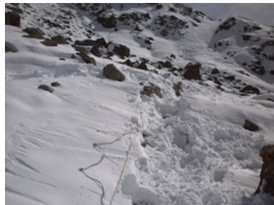
Fig.47: Measuring the profile length.
