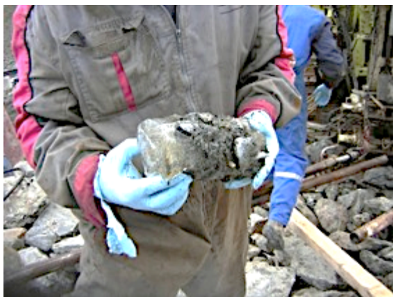
Fig. 83: Debris enriched ice core from drilling site #1.
