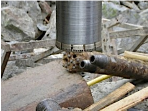
Fig. 81: Drill bit set with diamonds.
