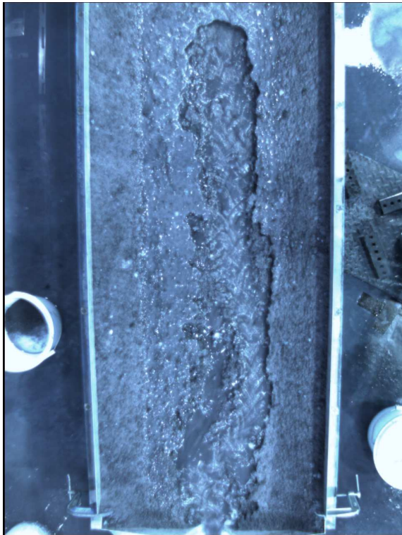
Fig. 24. The higher discharge causes less meandering morphology during the FDR
