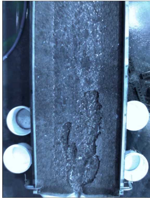
Fig. 19. Two channel arms develop due to back cut erosion
