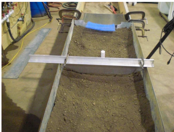
Fig. 9. FDR Soil Setup: rreparation of the soil surface by metal shape panel
