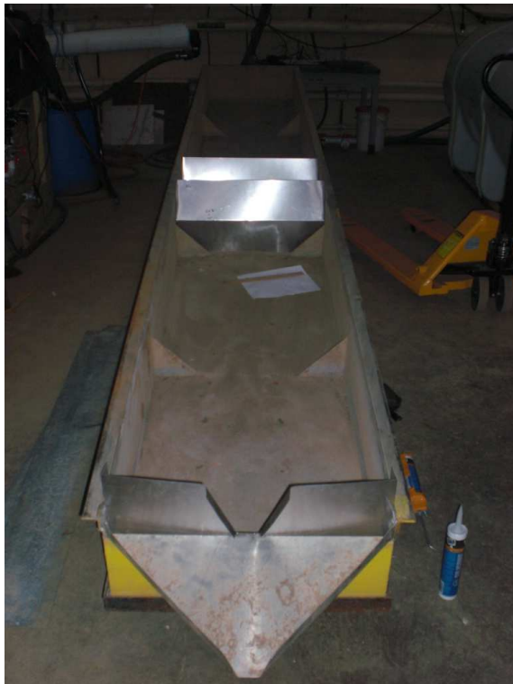
Fig. 5. Flume Setup: View into the plain steel flume
