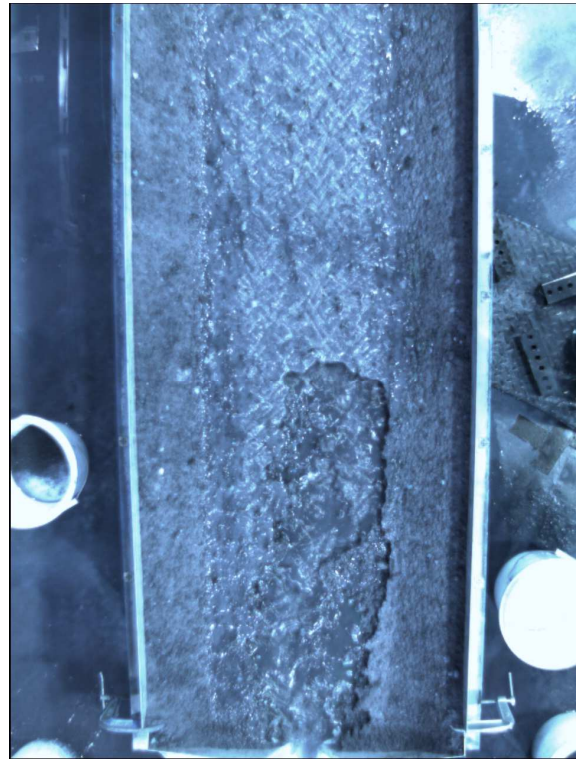
Fig. 23. Only one main channel occurs. The increase in discharge causes wider initial erosion
