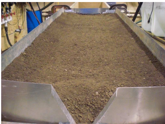
Fig. 11. Free Development Rill (FDR): soil preparation is uniform plain
