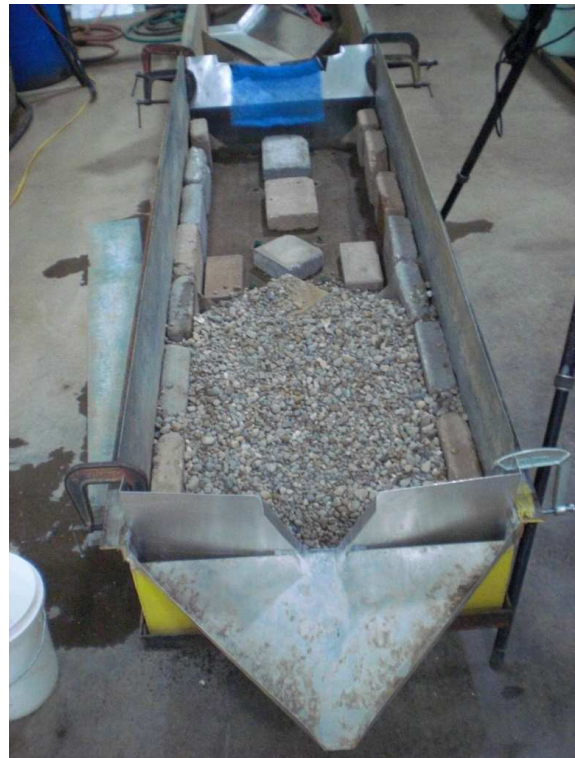
Fig. 6. Flume Setup Preparation: "Ground Drainage" layer (Gravel & Bricks)
