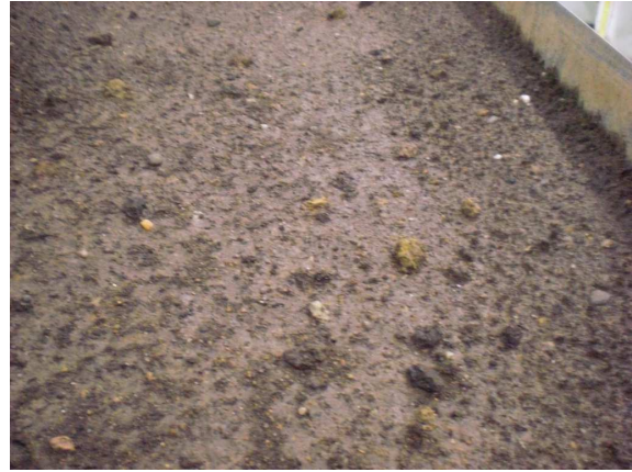
Fig. 14. Soil Pre Conditions: detail of the soil surface, smoothened and washed out relief – fine material clogs surface
