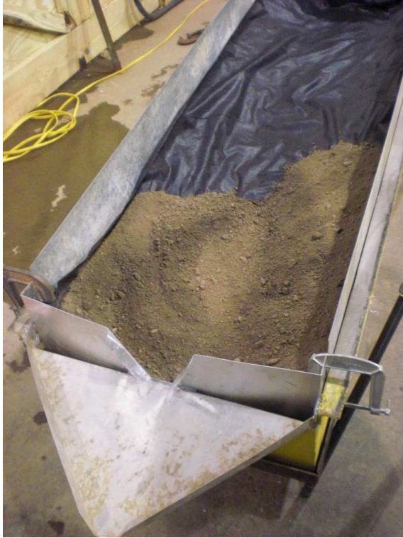
Fig. 7. Flume Setup Preparation: Soil layer with textile protection
