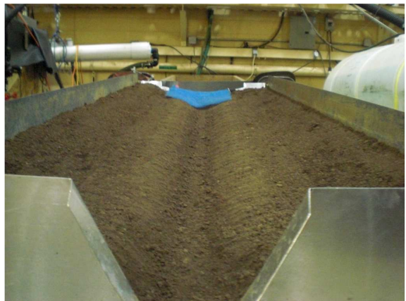
Fig. 12. Straight Constraint Rill (SCR): initial channel in the centre of the thalweg
