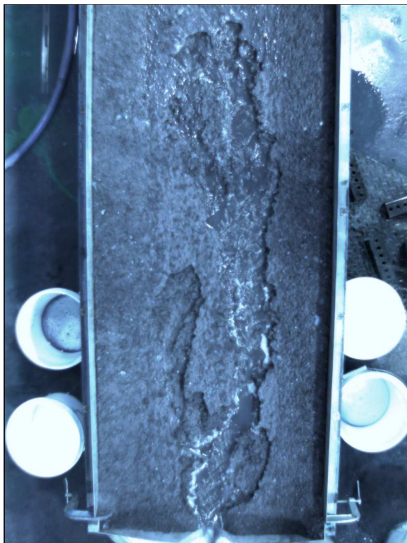
Fig. 20. One main channel formats whereas the Other side arm falls dry
