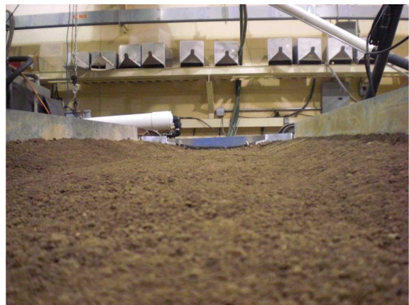
Fig. 10. View into the flume: the soil surface preparation is plain and rough by grain diameters
