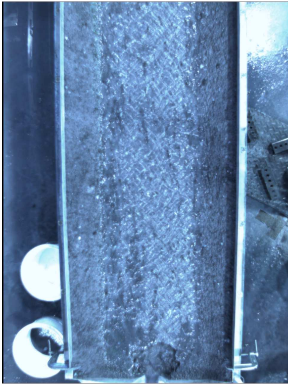
Fig. 22. Beginning stage of FDR 0,270 l/s: the shallow surface flow develops as a deeper water layer as in the 0,145 l/s experiment
