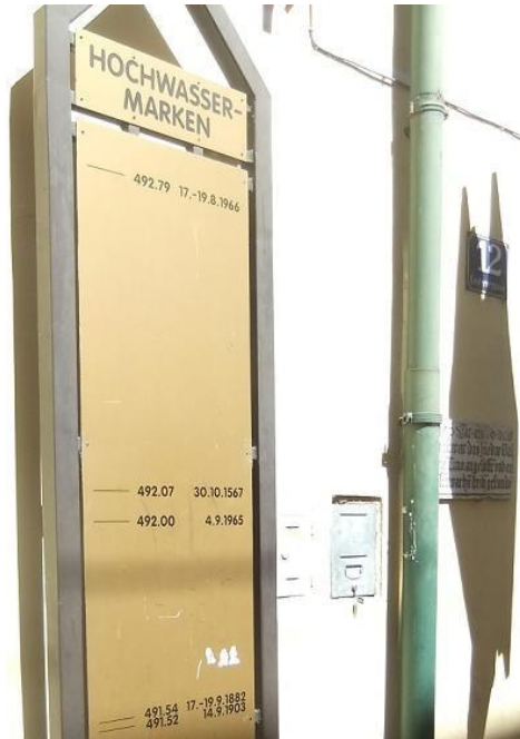
Figure 42: The flood elevation marks in Villach, Austria (elevation and year of the flood are known)
