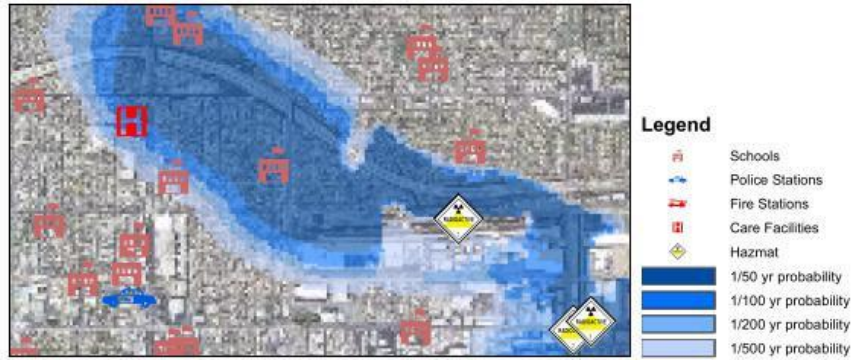
Figure 88: Flood extent map, produced with Hazus-MH Flood Model. Different flood extent periods are visualized in blue shade colours
