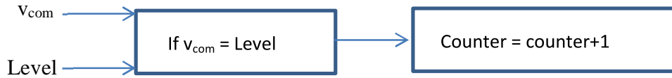
Figure 3: Counter to determine the presence of the particular voltage level in the common mode voltage using the Simulink model.
