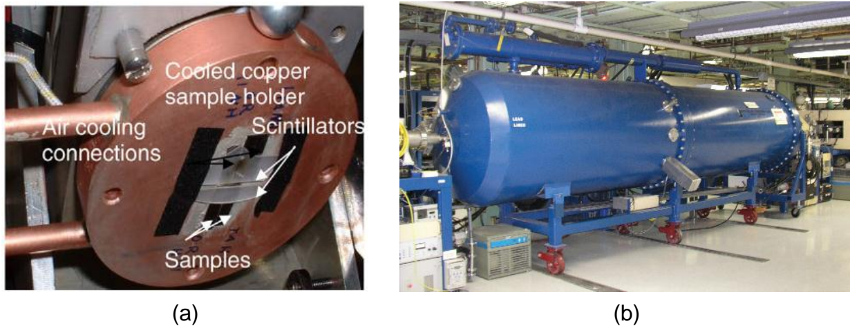
Figure 10. (a) Sample mounting in the ion beam irradiation experiment (26). (b) Tandem ion accelerator at IBML in LANL (24).
